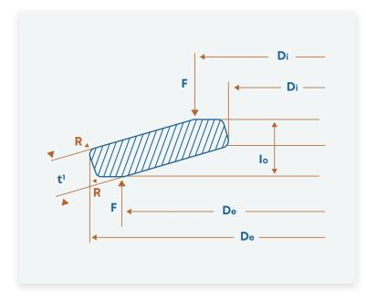
Group 3 disc springs have turned bearing surfaces and reduced disc thickness. The bearing surface increases the force, which is compensated for by the reduced disc thickness t'.
