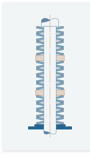
The figure above shows how a parallel stack can be converted into series stacks.
